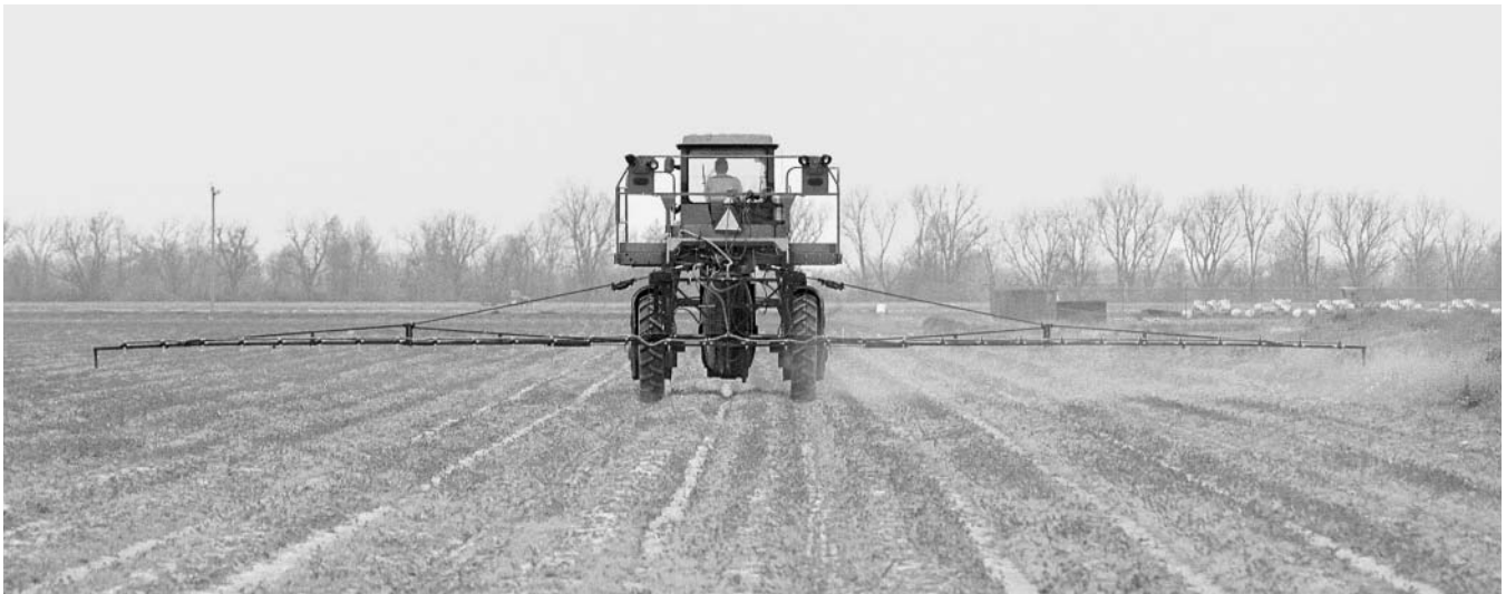
Figure 4. Application to bare ground showing greater drift from Extended Range 110015VS spray (right) than from Air Induction 110015VS spray nozzles (left).
